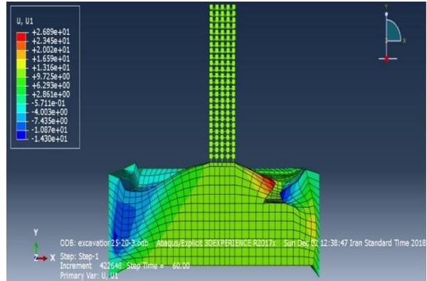
Displacement distribution in the 20-storey model at a distance of 20 m
