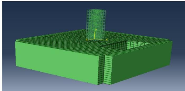
**Figure 2:** Position of the structure against the excavation edge
