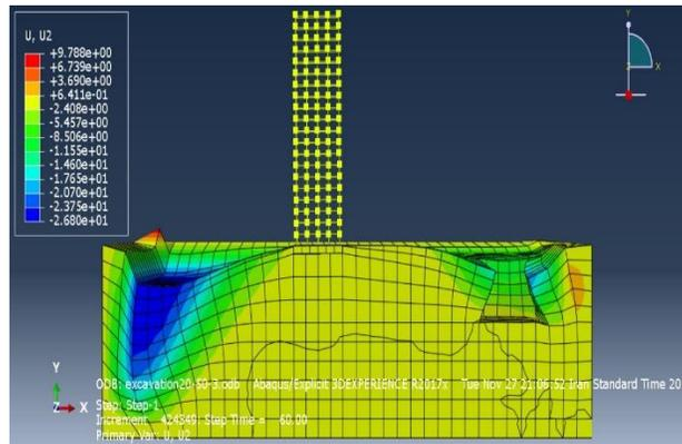
Displacement distribution in the 30-storey model at a distance of 50 m
