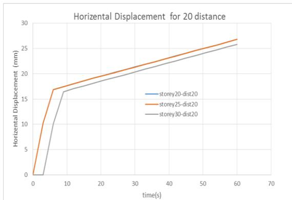
Horizontal displacement of excavation edge at a distance of 20 m
