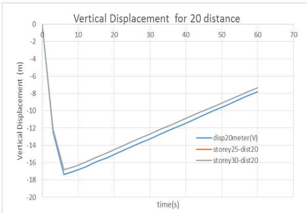
Vertical displacement of excavation edge at a distance of 20 m
