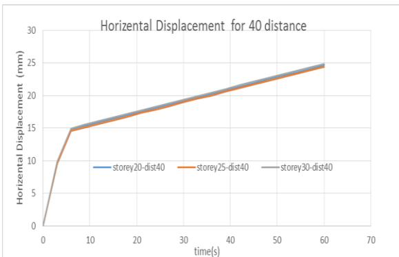
Horizontal displacement of excavation edge at a distance of 40 m
