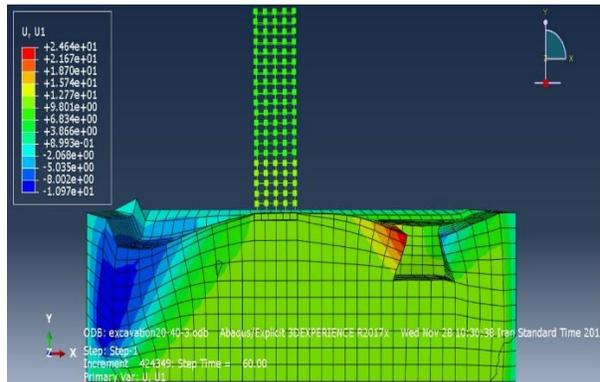
Displacement distribution in the 30-storey model at a distance of 20 m
