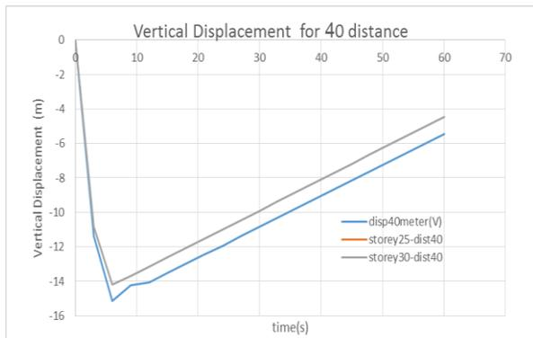
Vertical displacement of excavation edge at a distance of 40 m
