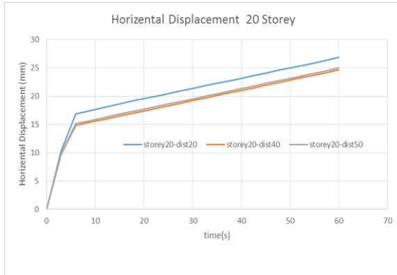
Horizontal displacement of excavation edge at a distance of 20 m
