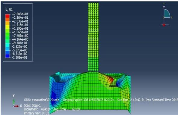
Displacement distributions in the 20-storey model at a distance of 40 m
