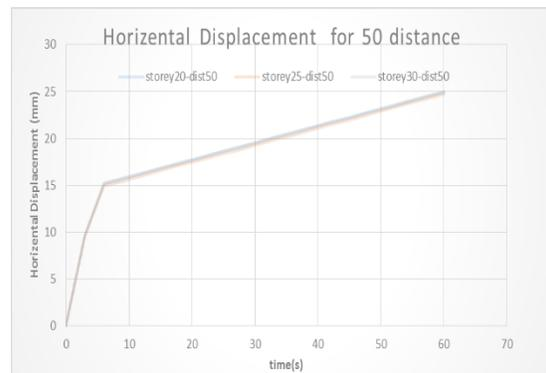
Horizontal displacement of excavation edge at a distance of 50 m
