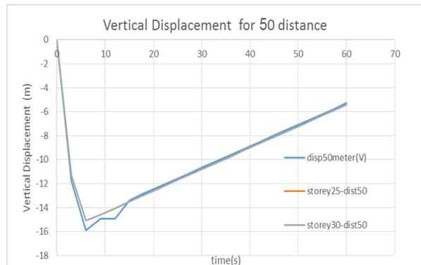
Vertical displacement of excavation edge at a distance of 50 m
