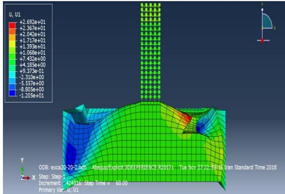
Displacement distribution in the 25-storey model at a distance of 20 m
