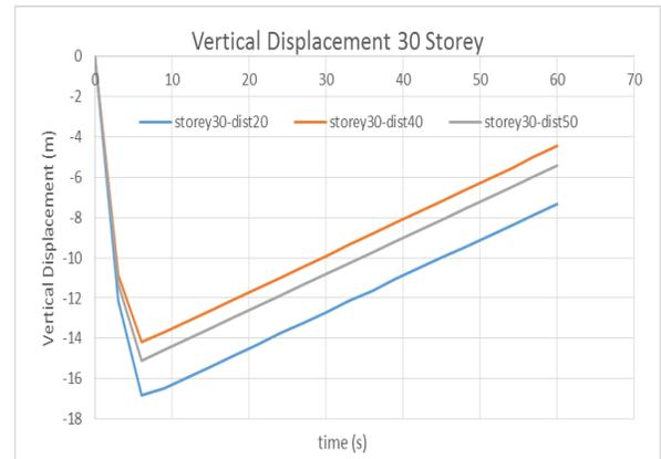
Vertical displacement of excavation edge at a distance of 30 m
