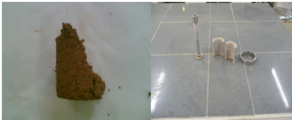
Figure1. Mold and hammer used to prepare the specimens Figure2. Broken cement specimen
