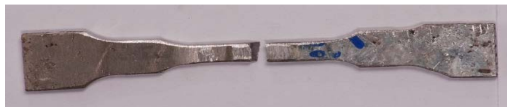
Figure 22: Upper and lower look of segment with speed of 12 cm/min prepared after tensile test
