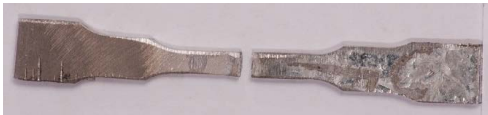
Figure 21: Upper and lower look of segment with speed of 10 cm/min prepared after tensile test
