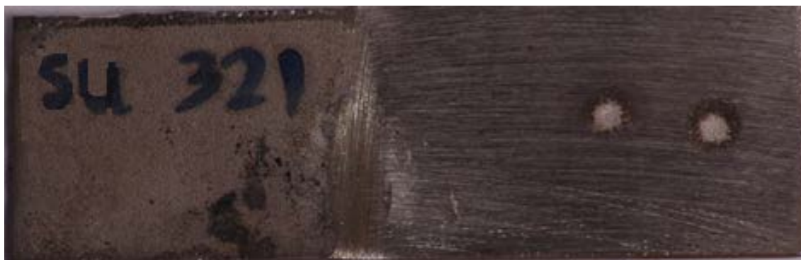
Figure 3: Look of segment of SU 321 tested for the analysis of chemical compound
