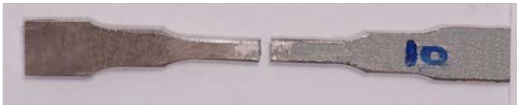
Figure 21: Upper and lower look of segment with speed of 10 cm/min prepared after tensile test
