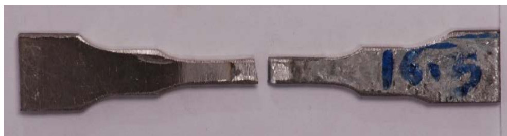
Figure 22: Upper and lower look of segment with speed of 12 cm/min prepared after tensile test
