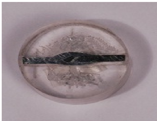
Figure 26: Mounted sample of microhardness testing
