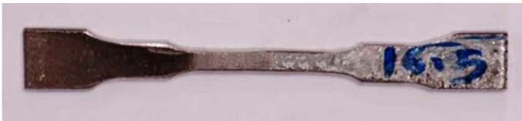
Figure 19: Upper look of segment with speed of 16 cm/min prepared before tensile test
