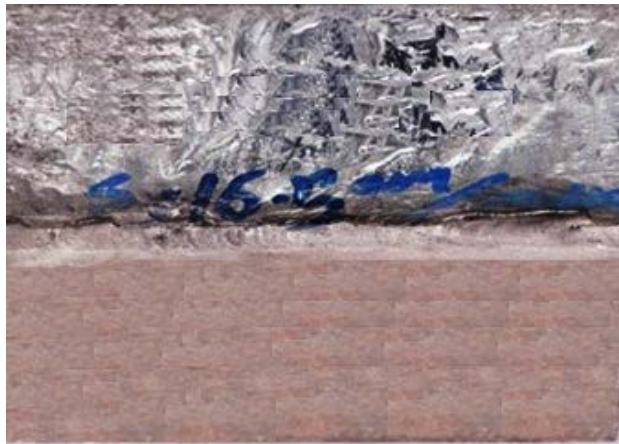
Figure 13: Segment welded from the head with with speed of 16.5cm/min, current intensity of 3mm 100A and filler of 3mm
