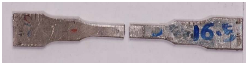
Figure 23: Upper and lower look of segment with speed of 16 cm/min prepared after tensile test
