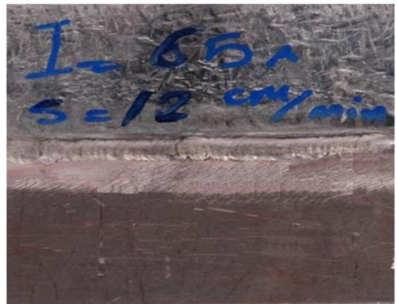
Figure 14: Segment welded from the head speed of 12cm/min, current intensity of 65A and filler
