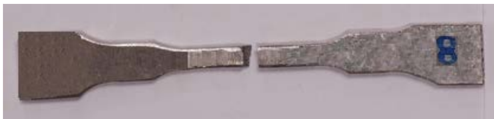
Figure 19: Upper look of segment with speed of 16 cm/min prepared before tensile test
