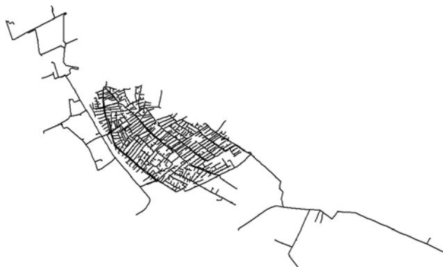
Figure 3: Single-line diagram of actual power network of Kar feeder of Kerman Province
