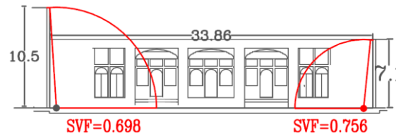
Figure 7. Sky view factor, southern view and other view in yard of Larry's house (source: Authors)
