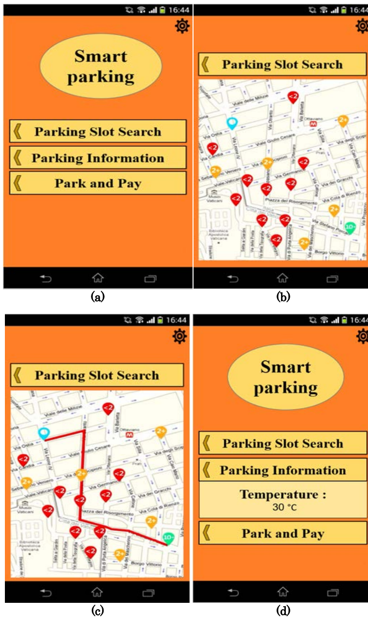
Figure 4: Android application of on-street smart parking a App Overview b The status of the parking slots in the city map c Route and the nearest roadway to the parking slot d Parking slots temperature information
