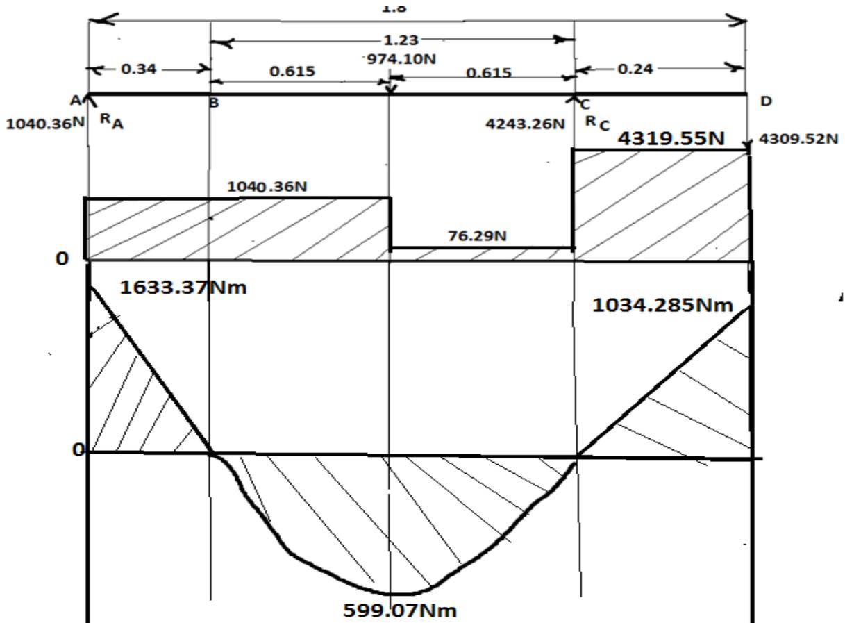
Fig 7. shear force and bending moment diagram
