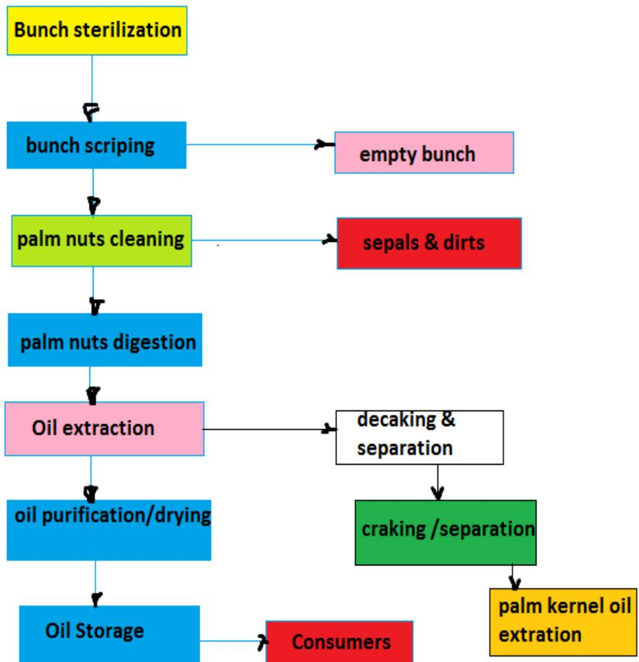
Figure 2: Flow diagram of palm oil extraction process
