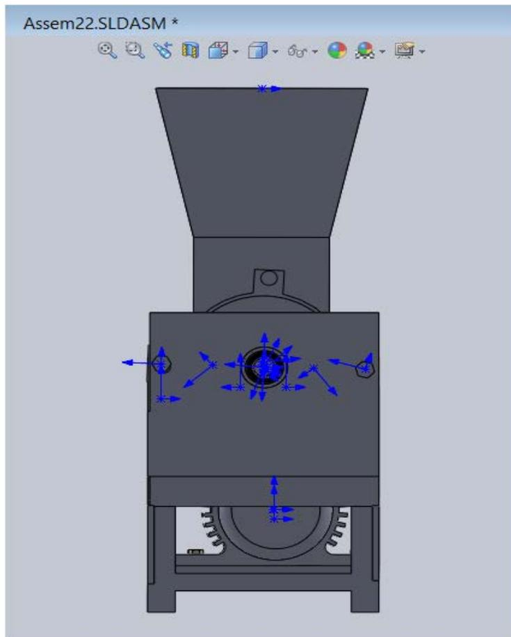
Fig 10. End View of the Continuous Palm Oil Fruits Digesting Machine
