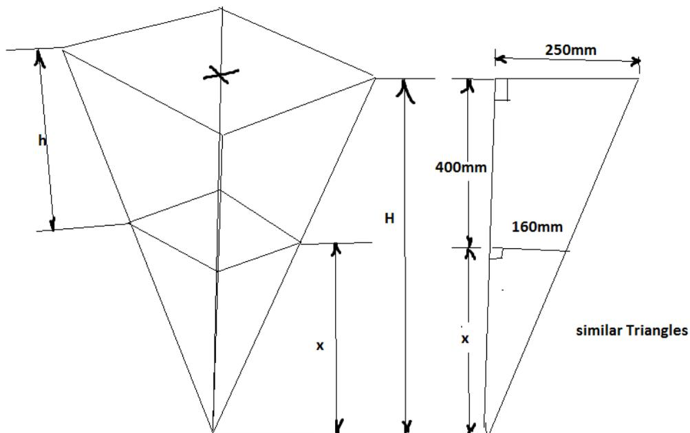
Fig.3a Pyramidal portion calculation using congruent triangle
