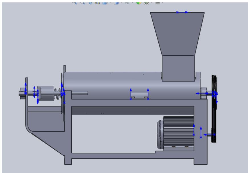
Fig 9. Side View of the Continuous Palm Oil Fruits Digesting Machine
