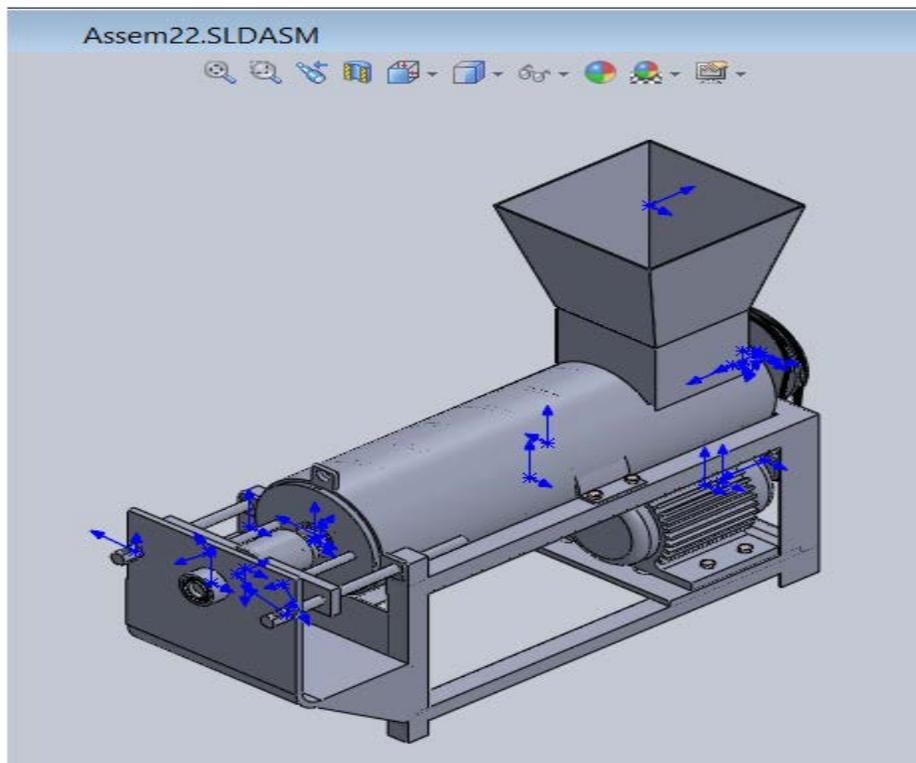
Fig 8. 3-D model of The continuous palm oil fruits digesting machine
