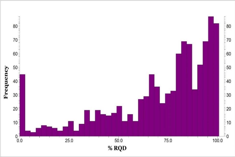
Figure 6– Frequency distribution of RQD values in geotechnical samples
