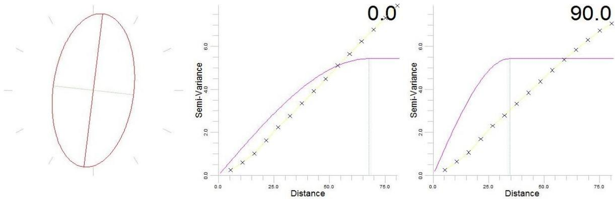
Figure 9– spherical variogram of Lugeon is almost the same in different directions and different range.
