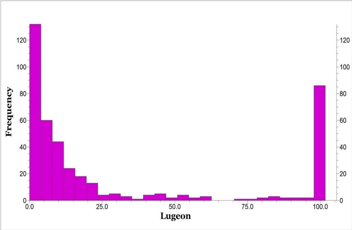
Figure 4– Frequency distribution of Lugeon values in the geotechnical samples
