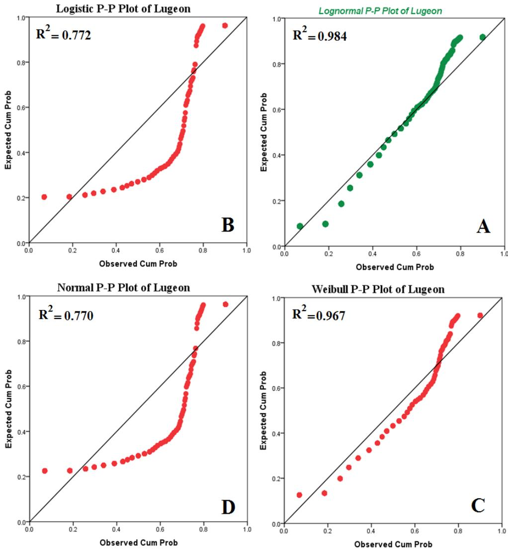
Figure 5– Comparison of the probability distribution for Lugeon data; (A) log-normal, (B) logistics, (C) Weibull, (D) normal. Lugeon values are highly adapted to the log-normal distribution function.
