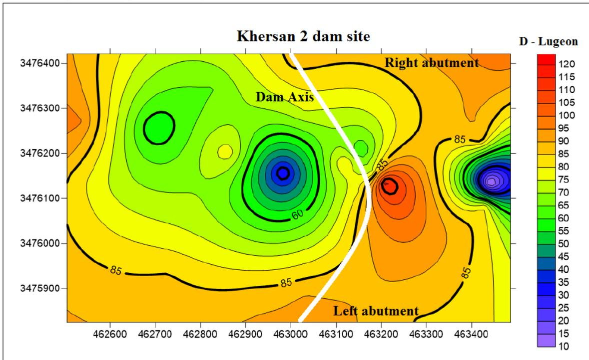
Figure 22–D Map (twice the standard deviation) for Lugeon
