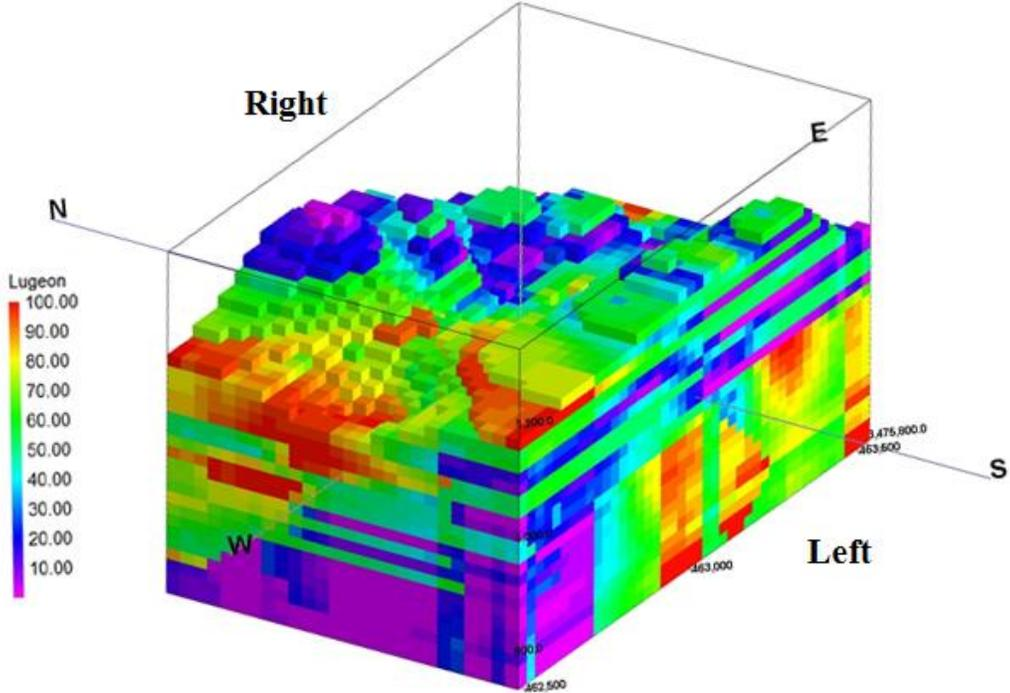
Figure 12- Three-dimensional model of the Lugeon status for the site under study
