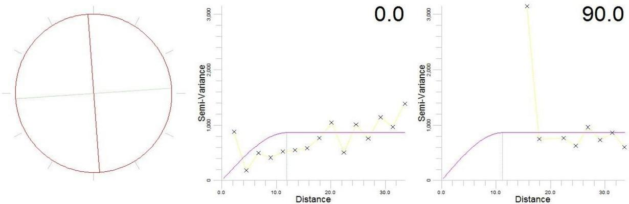
Figure 10– RQD spherical variogram is almost the same in different directions and different range
