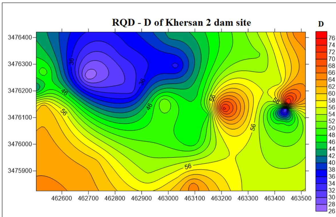
Figure 23–D Map (twice the standard deviation) of the RQD
