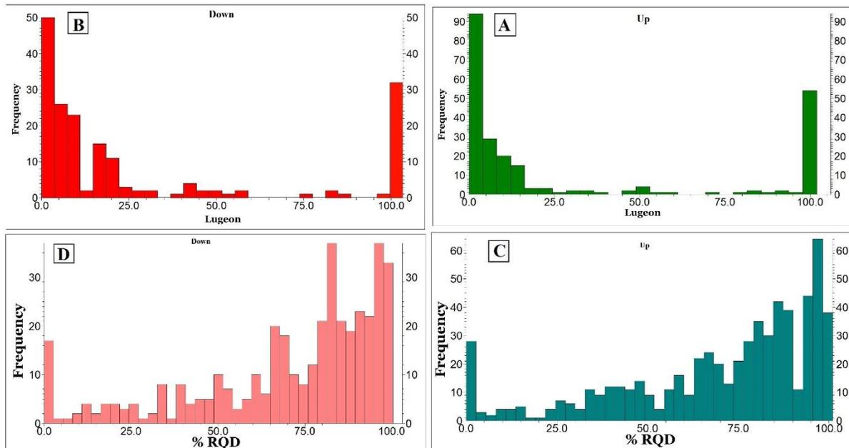
Figure 19: Frequency of Lugeon values in (A) upstream and (b) downstream and frequency of RQD values in (C) the upstream and (d) downstream of the dam
