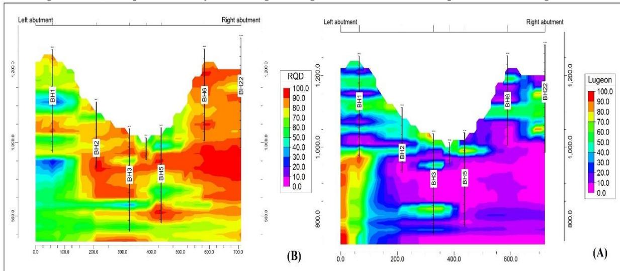
Figure 17– A cross-section of data (a) Lugeon and (b) RQD
