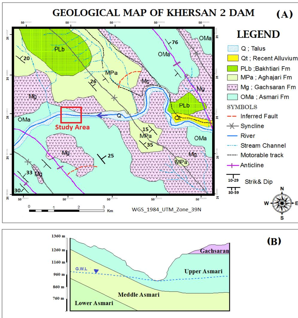
Figure 2– (A) Geological map, (B) geological cross-section of Khersan 2 dam site (Mahab Qods, 2010)
