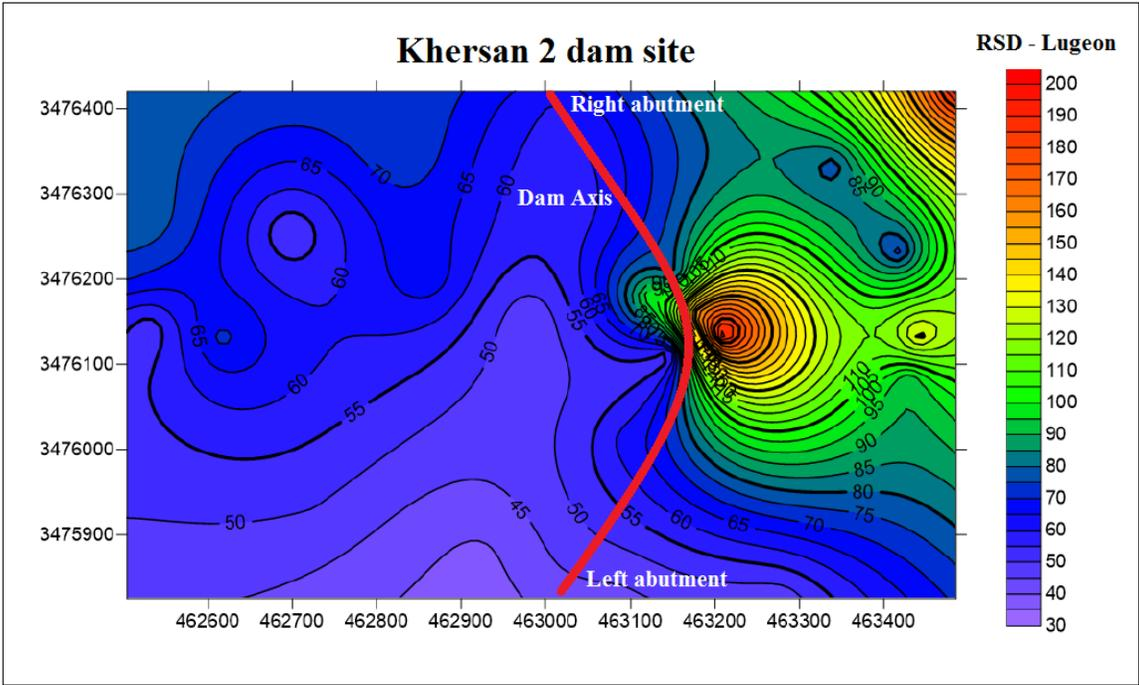
Figure 20– the map of relative standard deviation of Lugeon
