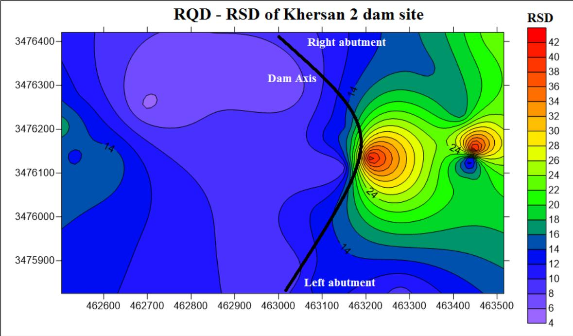
Figure 21–The relative standard deviation of the RQD
