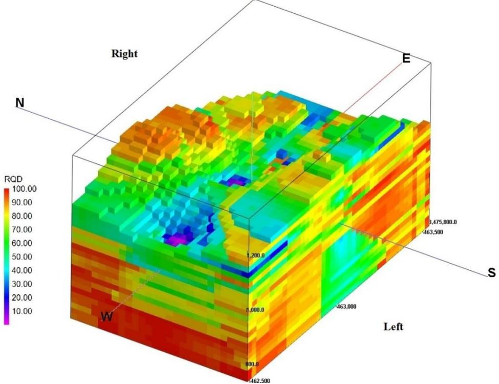
Figure 13- Three-dimensional model of the RQD status for the site under study
