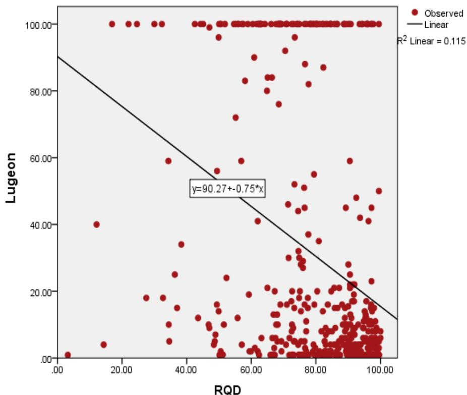
Figure 8– The diagram of correlation between Lugeon test results and RQD
