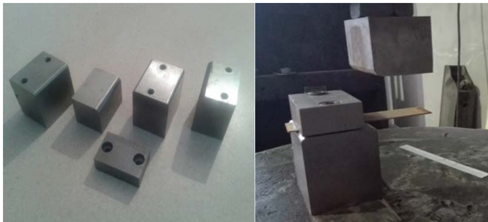
Figure 2: A schematic view of dies and how the test is done
