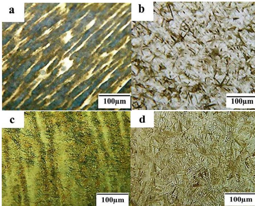
**Figure 4:** Optical micrographs of samples a) non-homogenized b) homogenized nESR steels. c) non-homogenized and d) homogenized ESR steels.
