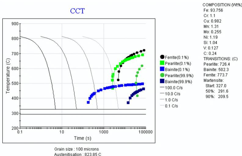
**Figure 3:** CCT diagram obtained using the JMAT PRO software for the studied steels.
