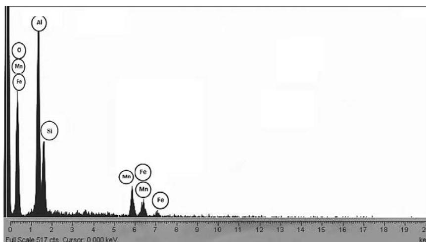
**Figure 2:** EDX analysis of inclusions in the nESR steel.
