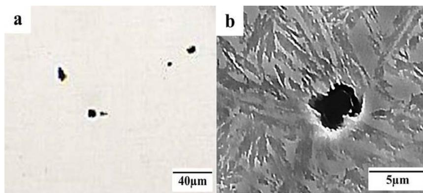
**Figure 1:** a) optical micrograph b) SEM micrograph of the inclusions.
