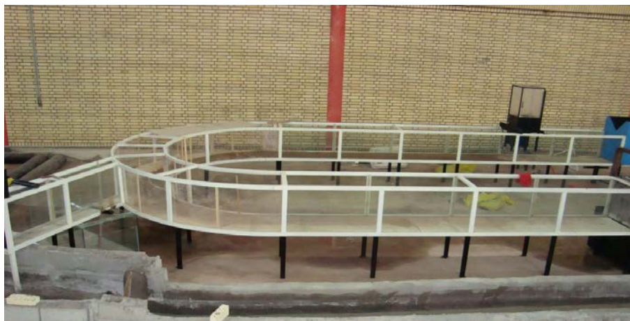
Figure 2 - Laboratory Flume Body
