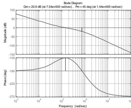
Fig. 2: Bode diagram of the PLL open loop transfer function
