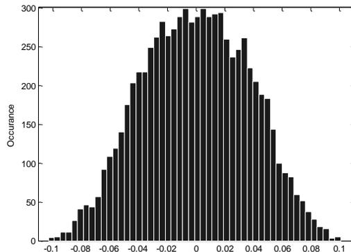
Fig. 11: Phase error histogram of a SQ\_EFM with n=19 bit and input =0.49
