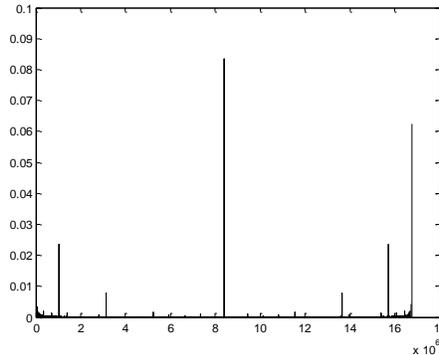
Fig. 9: Autocorrelation function of quantization error of a SQ\_EFM with  $n=19$  bit and  $\text{input}=2^{n/2}$
