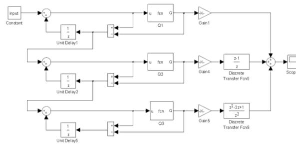
Fig. 3: Block diagram of MASH 1-1-1
