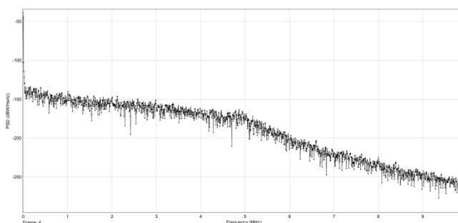
Fig. 14: Output spectrum of PLL with SQ\_MFFM
