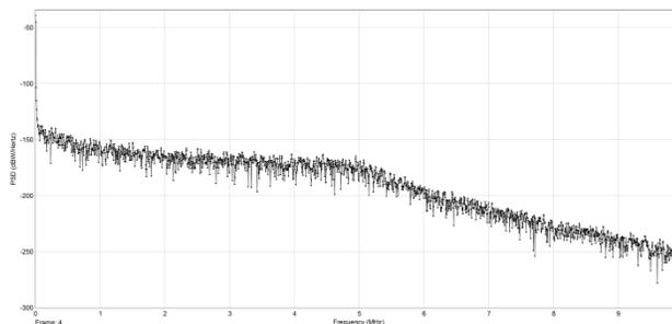
Fig. 13: Output spectrum of PLL with MASH 1-1-1
