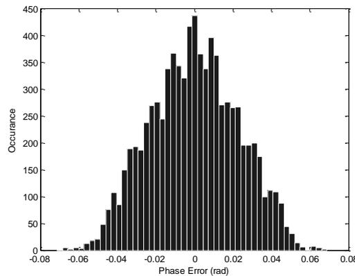
Fig. 12: Phase error histogram of a SQ\_MFFM with n=19 bit and input =0.49
