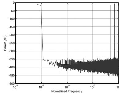
Fig. 7: PSD of MASH 1-1-1 with  $n=19$  and input  $=2^n/2$
