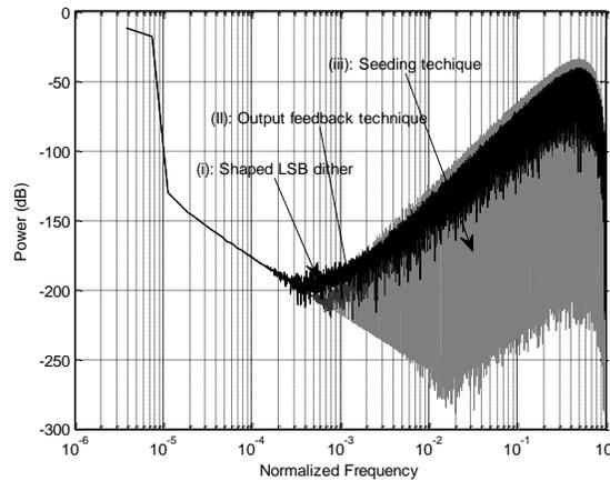
Fig. 8: PSD of a third order SQ\_EFM with  $n=13$  and input  $=2^n/2$ . The FFT length  $N_{FFT}=2^{18}$ ; (i) Shaped LSB dither, (ii) Output feedback technique and (iii) Seeding technique
