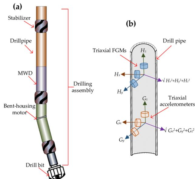
**Figure 1:** The directional module including the accelerometer and magnetometer in the measurement while-drilling tool of a drilling string
