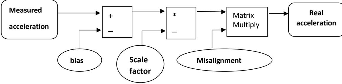
**Figure 2:** The accelerometer model block diagram
