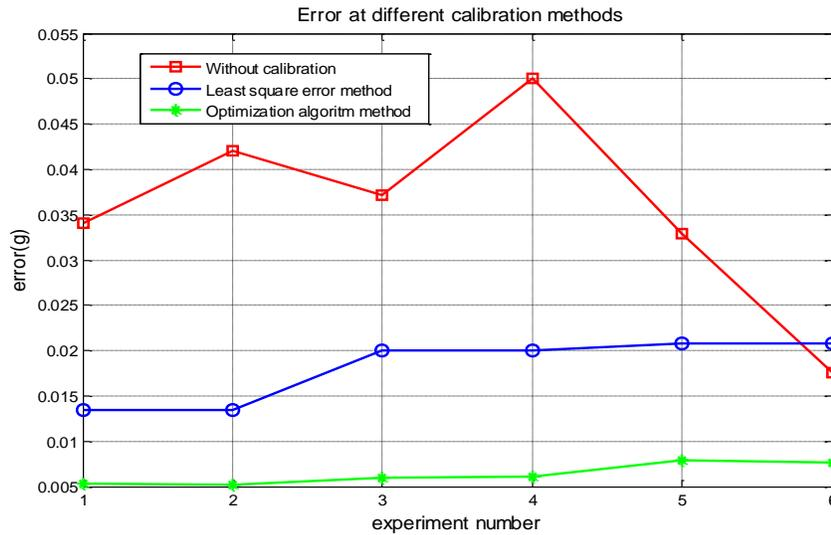
**Figure 3:** The comparison between the errors in different methods in several tests
