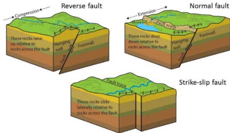
**Figure 1.** Normal, Reverse and Strike-slip Faults
