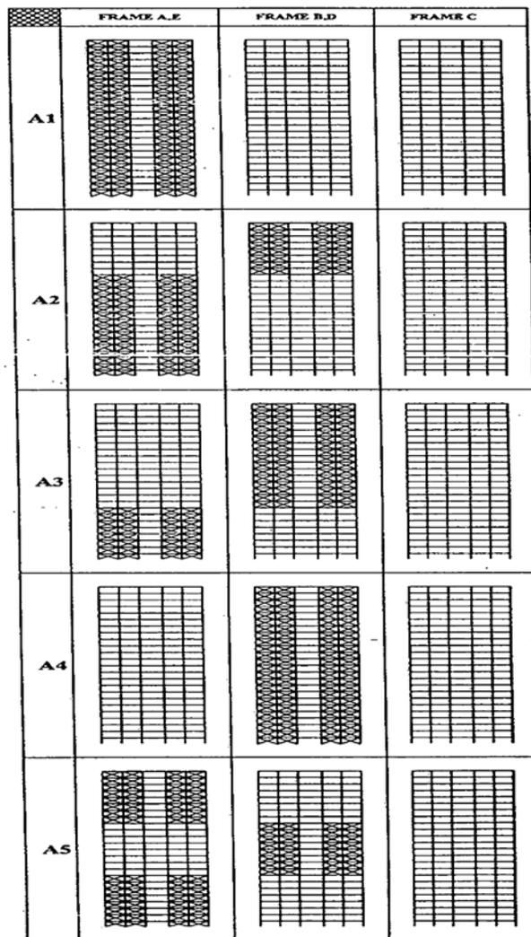
**Figure 1:** distribution of resistant lateral load-bearing elements in 24-storey buildings with 1:1 plan ratio (Group A)
