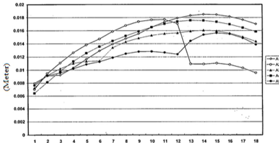
Figure 14: floors' relative drift in 18-storey models (group A)
