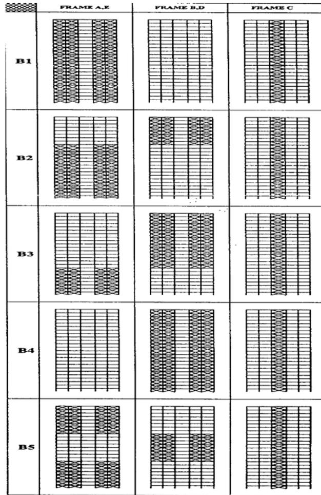
**Figure 2:** distribution of resistant lateral load-bearing elements in 24-storey buildings with 1:1 plan ratio (Group B)
