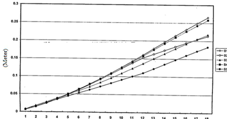
Figure 20: floors' displacement in 18-storey models (Group B)
