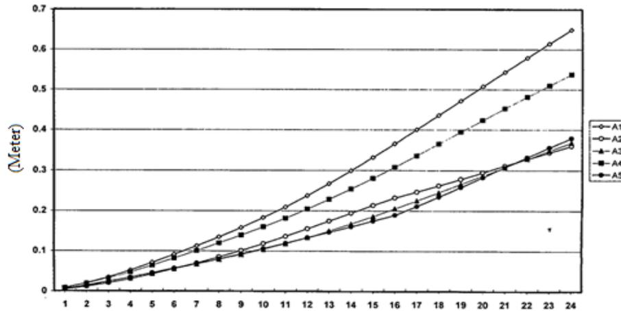
Figure 5: storeys' displacement in 24-storey models (Group A)
