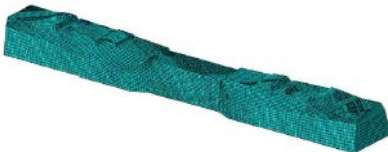
Figure 10. Meshing of a sleeper based on two-dimensional elements C3D8R and beam element B31
