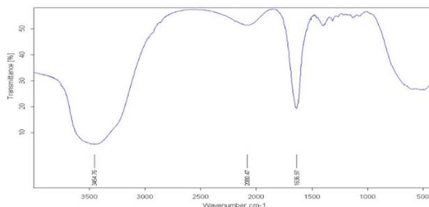
Figure 3: FT-IR spectrum of synthesized gold nanoparticles
