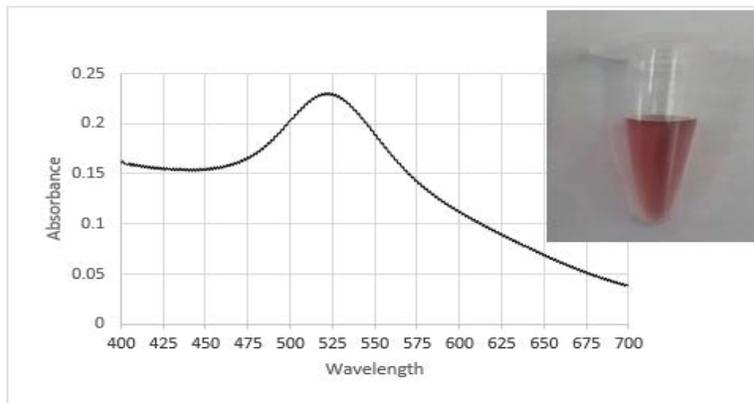
Figure 4: absorption spectrum of gold nanoparticles. As shown in the picture, the maximum absorption of gold nanoparticles occurred at the wavelength of 530 nm.
