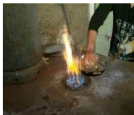
Image 28: Bleaching, tin spreading
