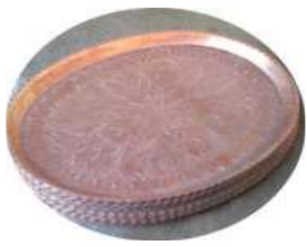
Image 13: Tray made by surfacing
