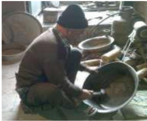
Image 17: Mesgari, hammering the base of the dish
