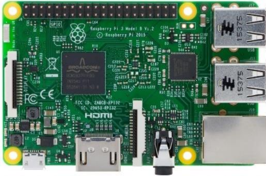
Figure 1: Picture of Raspberry Pi Model 3B used in the article
