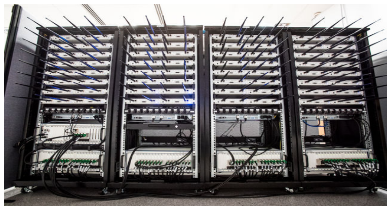
Figure 6. A base transceiver station with 128 antennas, manufactured by National Instruments Co. (NI)
