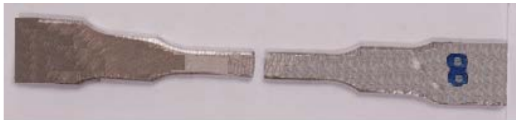
Figure 20: Upper and lower look of segment with speed of 8cm/min prepared after tensile test
