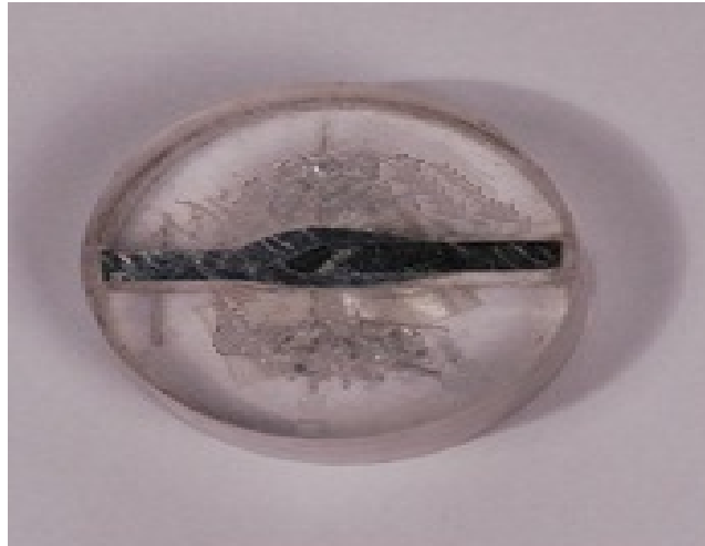
Figure 26: Mounted sample of microhardness testing
