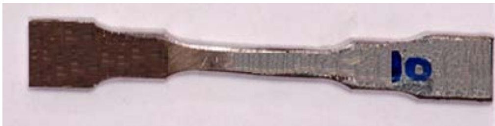
Figure 16: Upper look of segment with speed of 8cm/min prepared before tensile test
