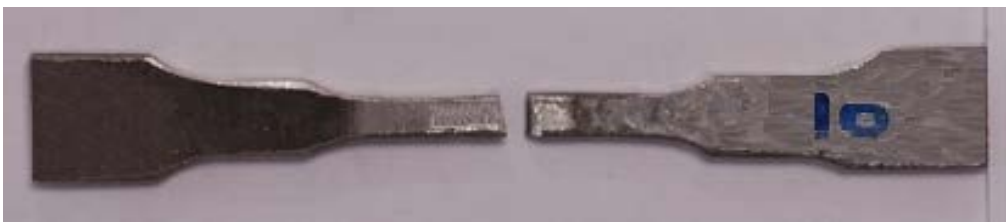
Figure 20: Upper and lower look of segment with speed of 8cm/min prepared after tensile test
