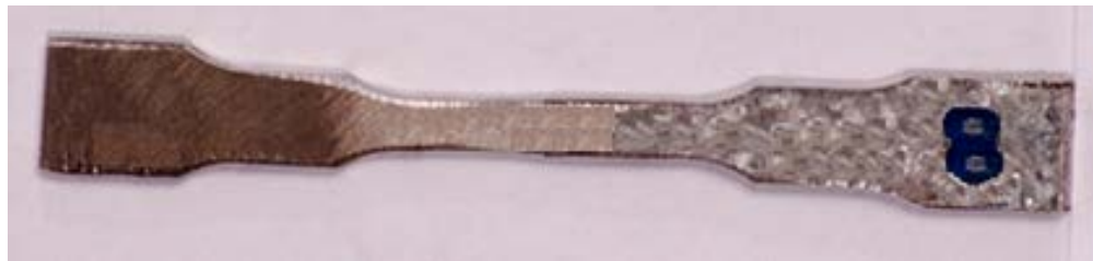
Figure 16: Upper look of segment with speed of 8cm/min prepared before tensile test
