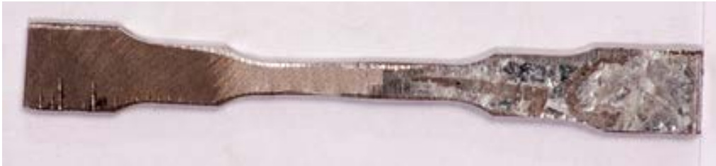
Figure 18: Upper look of segment with speed of 12 cm/min prepared before tensile test
