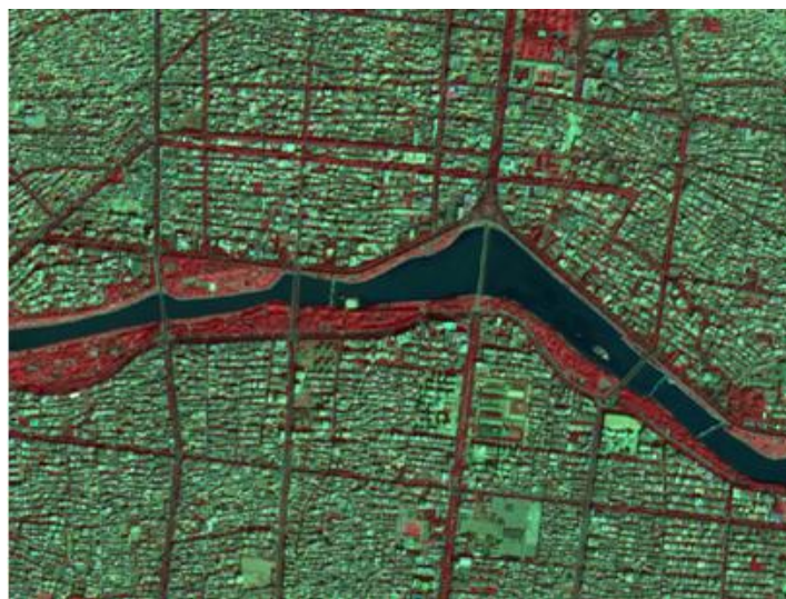
Figure 4: The merge of two data, P5 (CARTOSAT-I) satellite image with MX-LISS IV from P6
