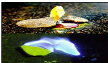
Figure 1: When burned, sulfur melts to a blood-red liquid and produces a blue flame that is clearly noticed in the dark (Wiberg, E. et al., 2001).
