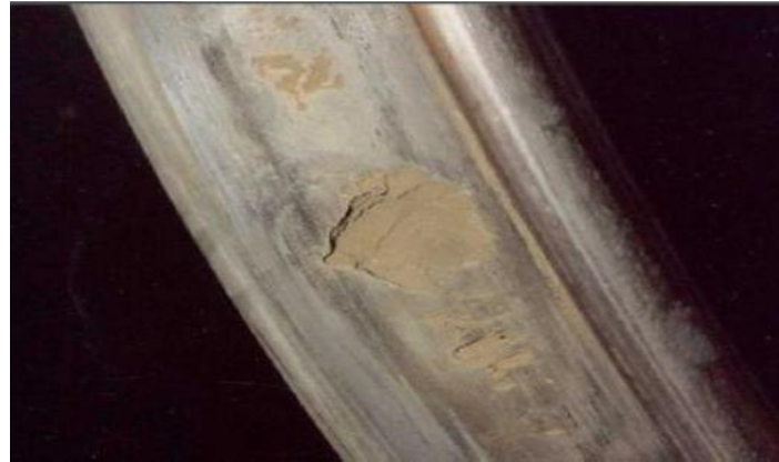
Figure 16: wear of wheel fatigue due to motion on the rail (Salehi and Afsharzadeh, "surface Metallurgy and Trilogy")
