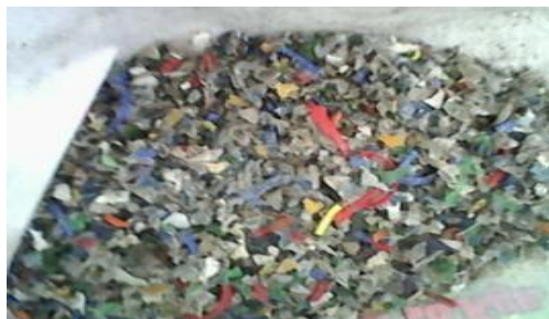
Plate 10: Pet Chips From Transparent Consumer’s Plastic Bottles
