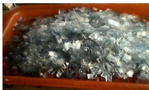
Plate 10: Pet Chips From Transparent Consumer’s Plastic Bottles
