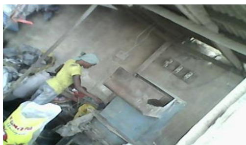
Plate 9: Grinding of Plastic Bottles in a Locally Fabricated Grinder
